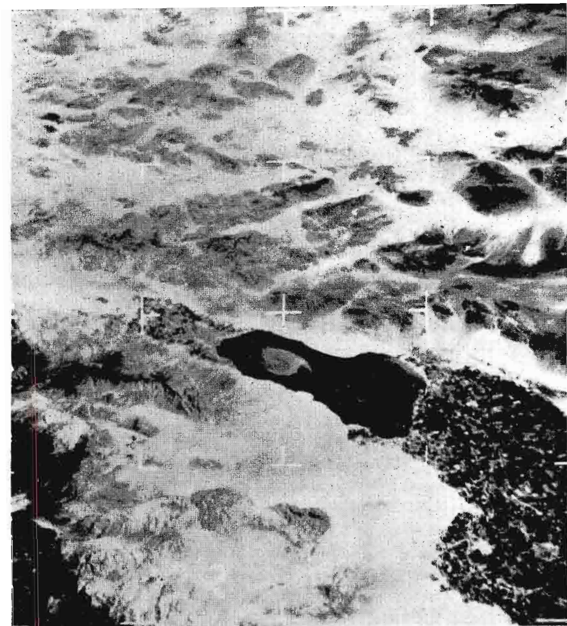
FIG. 2 This print of the Salton Sea was reproduced by a TV imaging system typical of those presently used in space. Resolution is approximately 800 TV lines.
