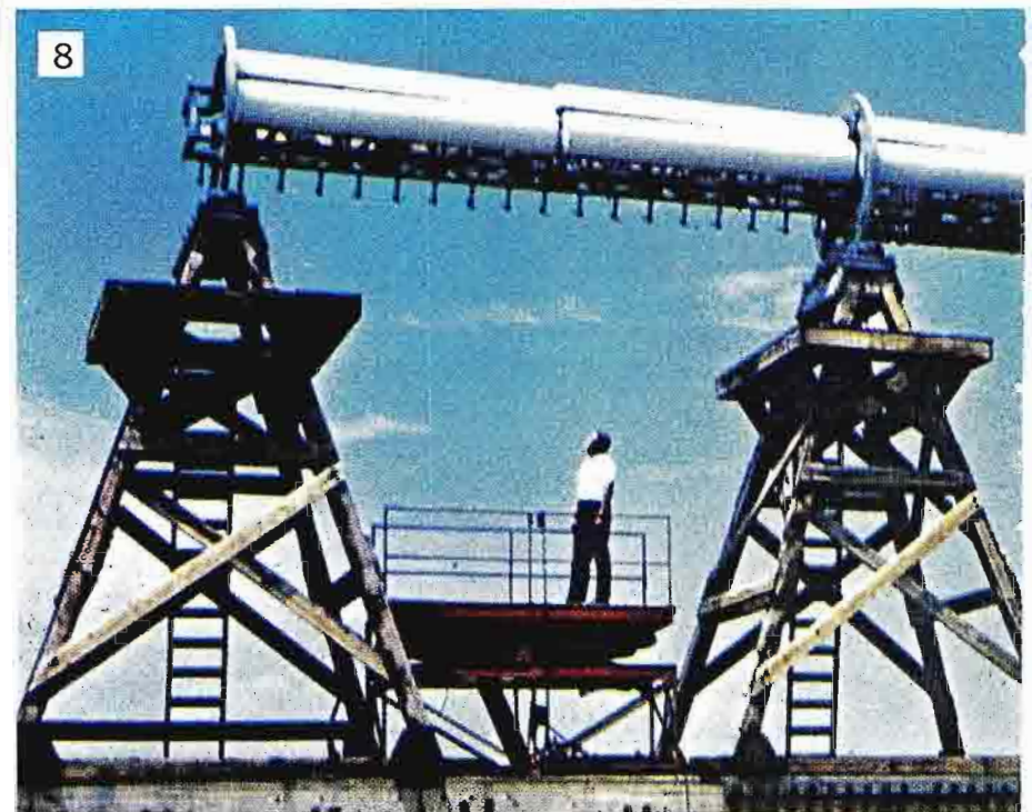
(8) Giant turntable called "Tiny Tim" where test antennas up to 15 tons move on a circular track 90 feet in diameter. It is one of three large turntables available for testing.
