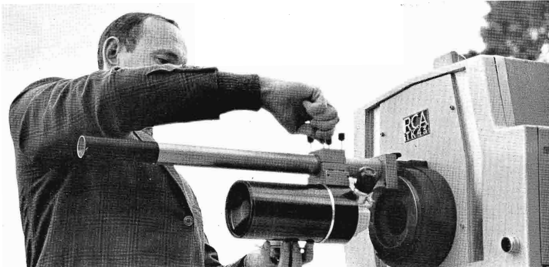
FIG. 6 Mounting the telescope—a compact casegrain type which is readily adaptable to the TK-43.
