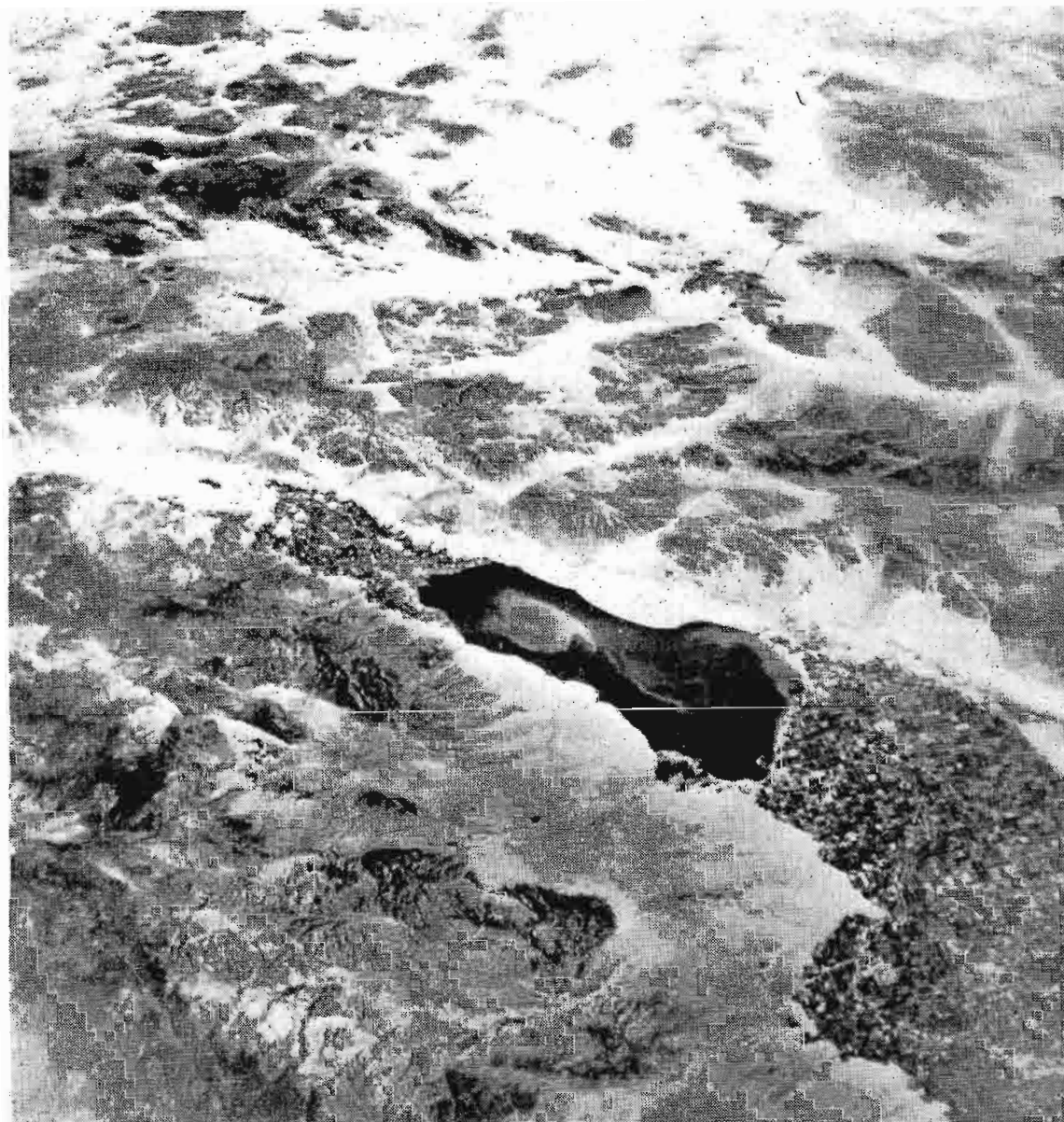
FIG. 3 This print of the Salton Sea was reproduced by the RCA Two-Inch Return Beam Vidicon-Laser Beam Image Reproducer. Resolution is in the order of 5000 TV lines.
